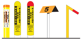
Examples of pipeline markers
